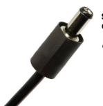
SLIDE THE HEATSHRINK ONTO THE CONNECTOR **LEAVING AN EQUAL** OVERLAP AT EACH END
